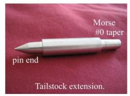
**Fig. 3:** Left) "Reduced-length" Morse #0 taper shape typically used on a tabletop lathe. Right) Dead center Morse Adapter, perhaps the simples appliation of the LASER protractor.
